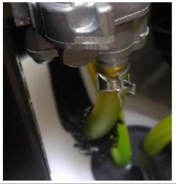
3. Locate the 'internal' fuel line on the Fuel Valve Kit (has a male barb fitting).
