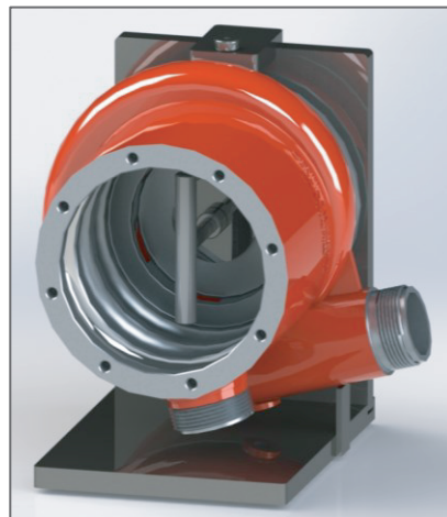
Figure 6: Slide in Drilling Guide and secure pump body by tightening T-bolt
