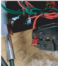
Install newly crimped connectors onto the toggle switch tabs (as shown).
