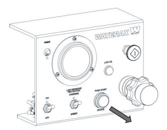
2. Install the new toggle switch as shown.
