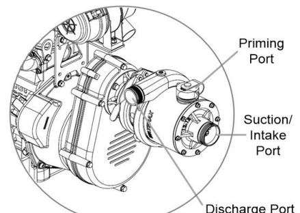
! **DO NOT** run engine with pump disconnected.
