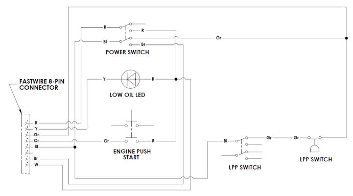
The following schematic is to represent the wiring harness going from the MCP to the pump unit.
