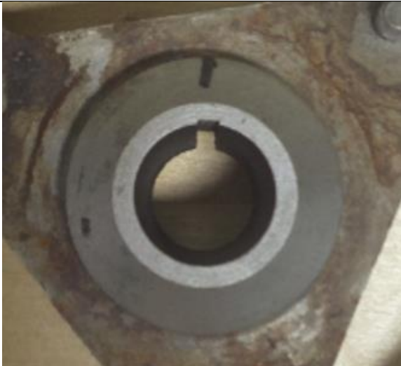
Old flywheel: no recess on center hub
