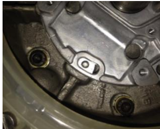
Stator plate adjustment, 1-1.5 mm CCW
