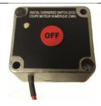
Remove the back lid (two flat head Phillips screws) to access the dipswitches.
