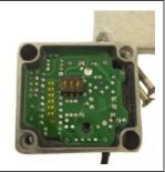
Using a small flat screw driver, gently flip up the third switch to the "ON" position. This will set the cut-off speed to the highest setting.
