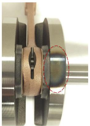
This heat treatment discoloration is normal and happens during the induction hardening process. The discoloration has **no impact** on the crankshaft.
