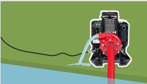
Keep priming until either there is water coming out of the discharge or out of the spout on the hand primer.
