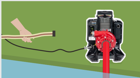
Attach the discharge hose. Once again, it is important to have an airtight connection.
