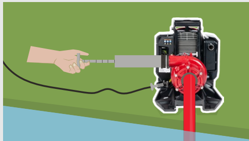
Priming the pump end can be done by either agitating the foot valve or by using a hand primer.
